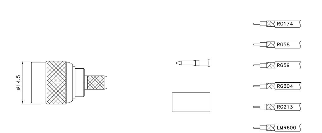
CENTER PIN GOLD PLATING 3µ THICK OVER NICKEL PLATING 70µ THICK OVER NICKEL STRIKE
