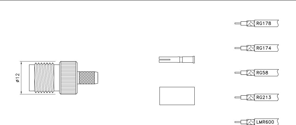
CENTER PIN GOLD PLATING 3µ THICK OVER NICKEL PLATING 70µ THICK OVER NICKEL STRIKE
