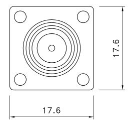
CENTER PIN GOLD PLATING 3µ THICK OVER NICKEL PLATING 70µ THICK OVER NICKEL STRIKE
