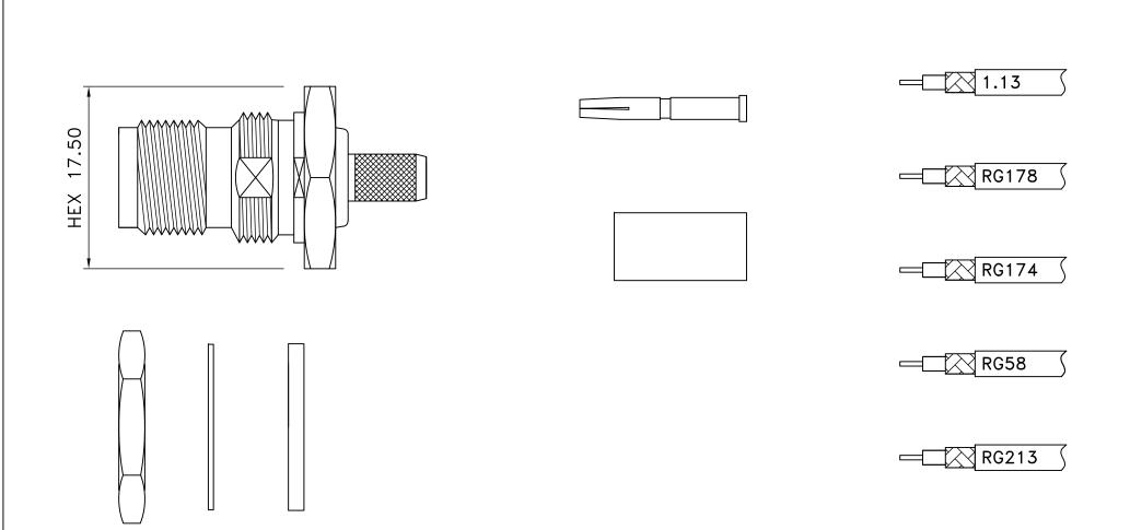
CENTER PIN GOLD PLATING 3µ THICK OVER NICKEL PLATING 70µ THICK OVER NICKEL STRIKE
