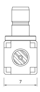
CENTER PIN GOLD PLATING 1.5µ THICK OVER NICKEL PLATING 70µ THICK OVER NICKEL STRIKE
