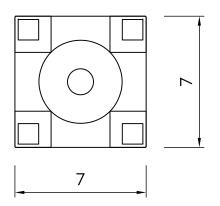
CENTER PIN GOLD PLATING 20µ THICK OVER NICKEL PLATING 70µ THICK OVER NICKEL STRIKE
