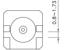
CENTER PIN GOLD PLATING 20µ THICK OVER NICKEL PLATING 70µ THICK OVER NICKEL STRIKE
