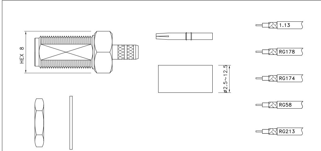
CENTER PIN GOLD PLATING 20µ THICK OVER NICKEL PLATING 70µ THICK OVER NICKEL STRIKE
