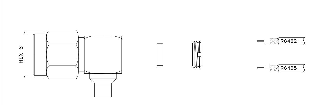
CENTER PIN GOLD PLATING 20µ THICK OVER NICKEL PLATING 70µ THICK OVER NICKEL STRIKE
