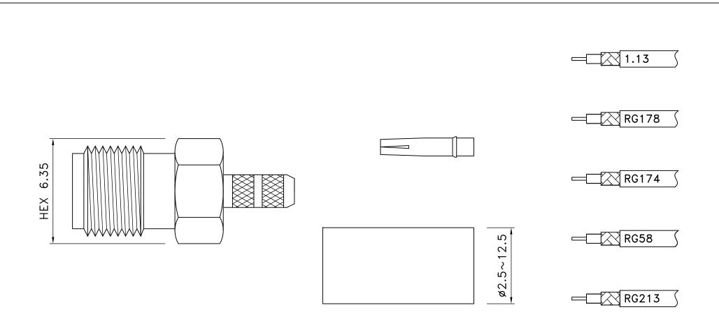
CENTER PIN GOLD PLATING 20µ THICK OVER NICKEL PLATING 70µ THICK OVER NICKEL STRIKE
