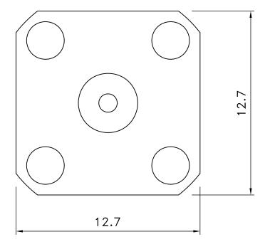
CENTER PIN GOLD PLATING 20µ THICK OVER NICKEL PLATING 70µ THICK OVER NICKEL STRIKE
