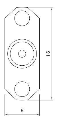
CENTER PIN GOLD PLATING 20µ THICK OVER NICKEL PLATING 70µ THICK OVER NICKEL STRIKE
