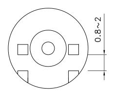
CENTER PIN GOLD PLATING 20µ THICK OVER NICKEL PLATING 70µ THICK OVER NICKEL STRIKE
