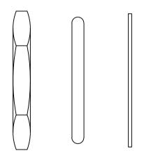
CENTER PIN GOLD PLATING 3µ THICK OVER NICKEL PLATING 70µ THICK OVER NICKEL STRIKE BODY NICKEL PLATING 70µ THICK OVER NICKEL STRIKE BRASS AND PTFE PER SGS FINISH PLATING THICKNESS IN MICRO-INCHES COPPER PARTS AUTOMATIC CNC MANUFACTURING
