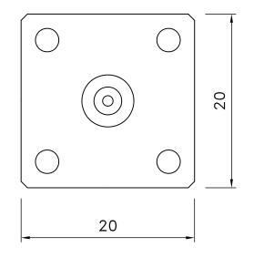
CENTER PIN GOLD PLATING 3µ THICK OVER NICKEL PLATING 70µ THICK OVER NICKEL STRIKE BODY NICKEL PLATING 70µ THICK OVER NICKEL STRIKE BRASS AND PTFE PER SGS FINISH PLATING THICKNESS IN MICRO-INCHES COPPER PARTS AUTOMATIC CNC MANUFACTURING
