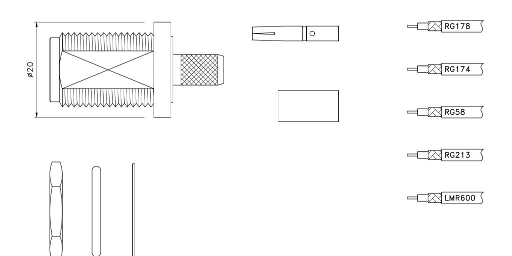
CENTER PIN GOLD PLATING 3µ THICK OVER NICKEL PLATING 70µ THICK OVER NICKEL STRIKE BODY NICKEL PLATING 70µ THICK OVER NICKEL STRIKE BRASS AND PTFE PER SGS FINISH PLATING THICKNESS IN MICRO-INCHES COPPER PARTS AUTOMATIC CNC MANUFACTURING
