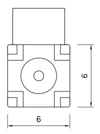
CENTER PIN GOLD PLATING 20µ THICK OVER NICKEL PLATING 70µ THICK OVER NICKEL STRIKE
