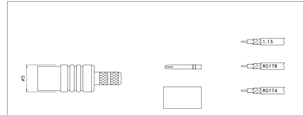
CENTER PIN GOLD PLATING 20µ THICK OVER NICKEL PLATING 70µ THICK OVER NICKEL STRIKE
