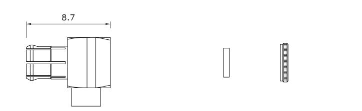
CENTER PIN GOLD PLATING 30µ THICK OVER NICKEL PLATING 70µ THICK OVER NICKEL STRIKE
