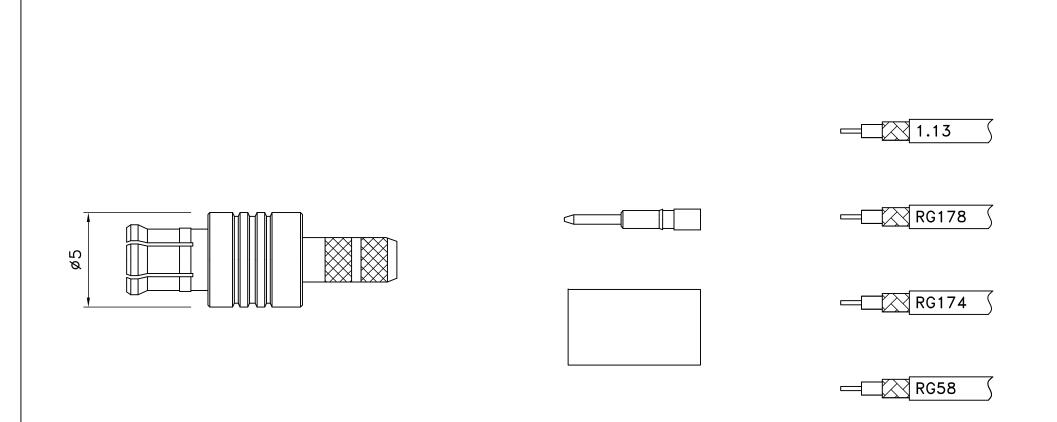
CENTER PIN GOLD PLATING 20µ THICK OVER NICKEL PLATING 70µ THICK OVER NICKEL STRIKE
