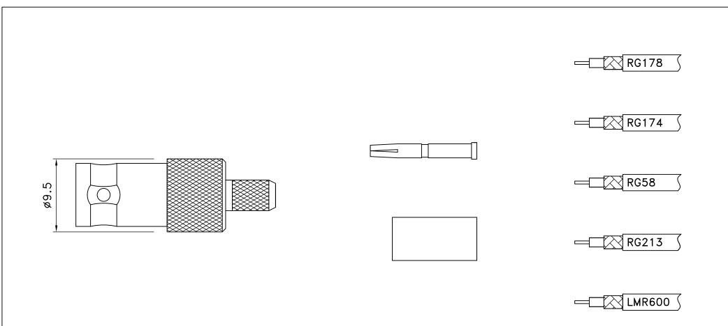
CENTER PIN GOLD PLATING 3µ THICK OVER NICKEL PLATING 70µ THICK OVER NICKEL STRIKE
